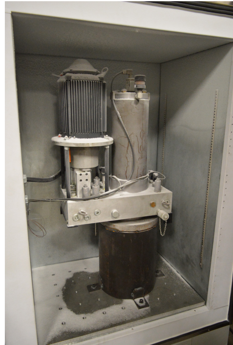
E 2 H low temperature test in Cowan's R&D lab
